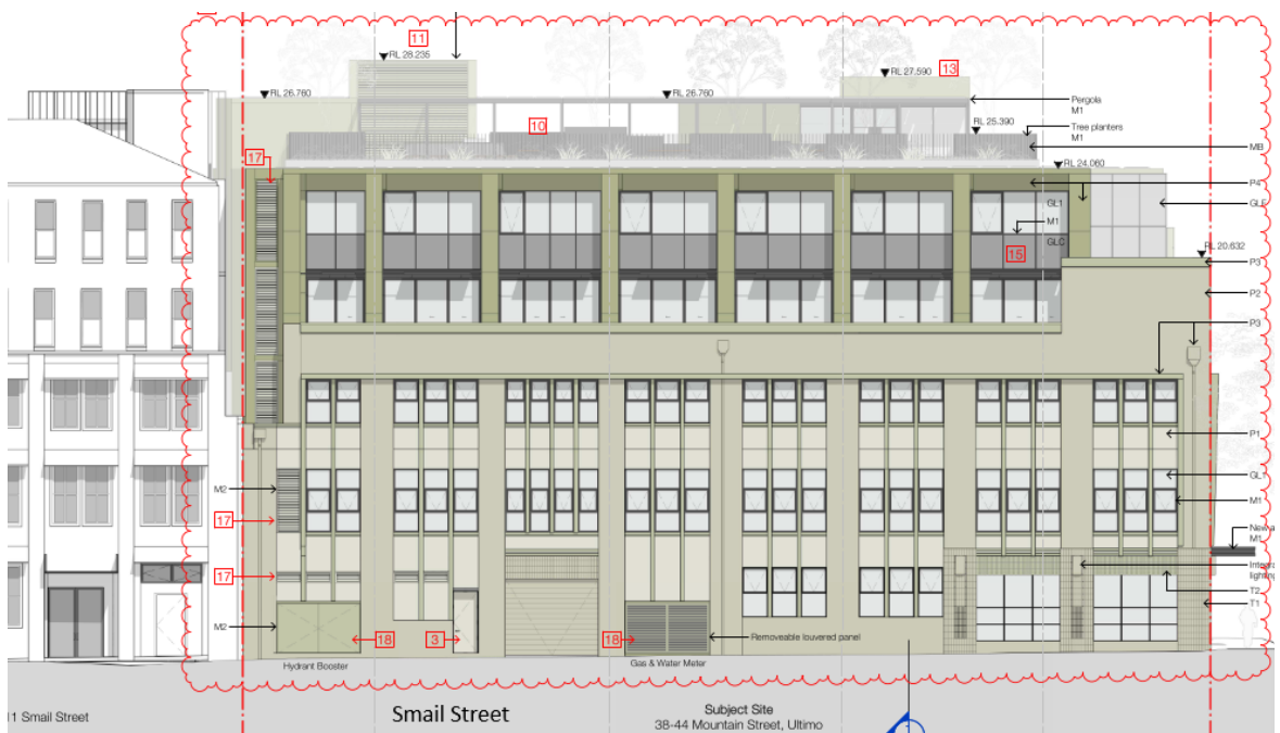
Figure 23: Proposed north elevation, with lift overrun shown top right, and proposed cooling tower shown top left
